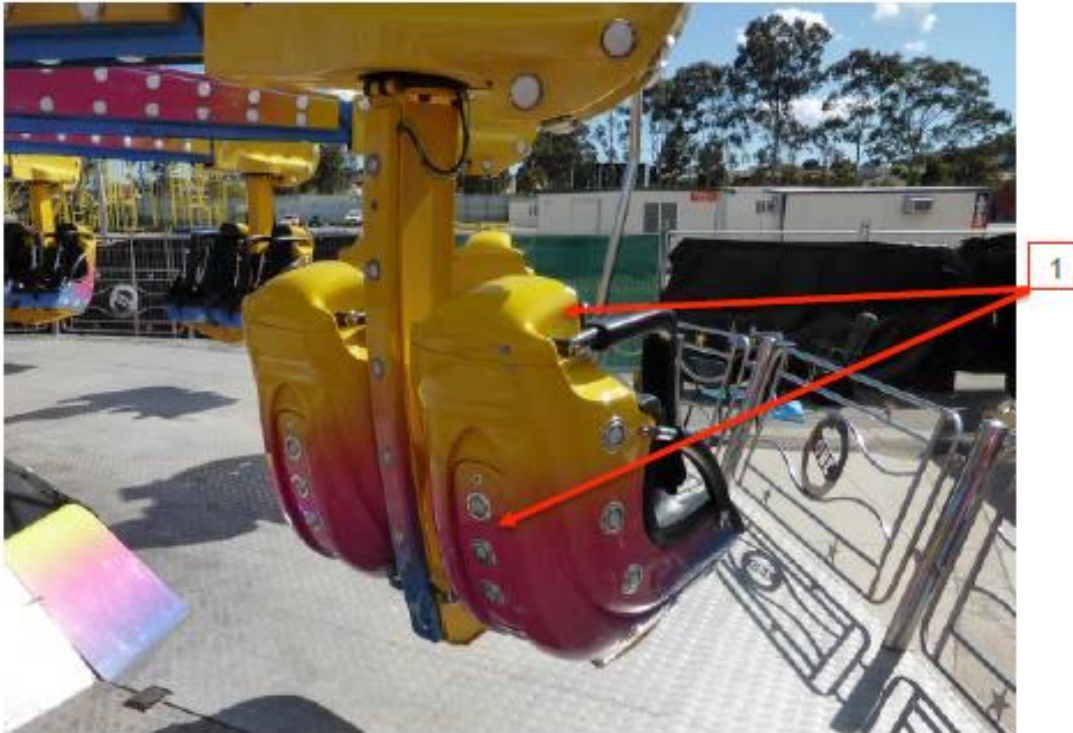
Figure 8 Airmaxx 360 Carriage showing access covers on seat in place (P1010258.JPG)
