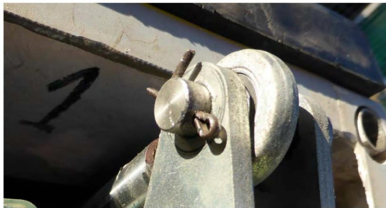
Figure 39 Airmaxx 360 Damaged split pin (P1010479.JPG)
