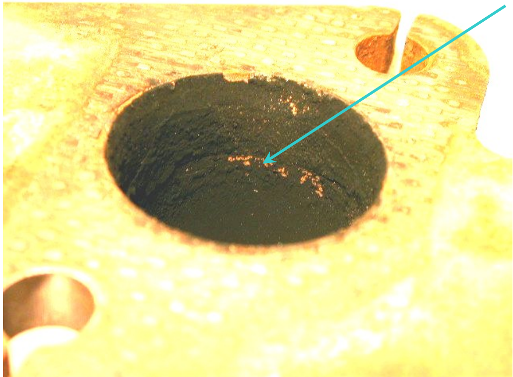
Figure 3 Internal view of extractor pipe at engine flange showing carbon coating and pipe cracking (arrow).
