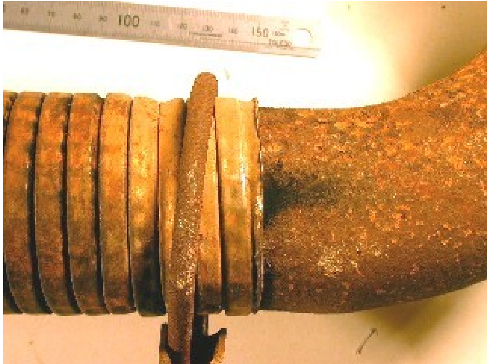
Figure 8 Detail of exhaust pipe and flexible tube connection showing carbon deposits.
