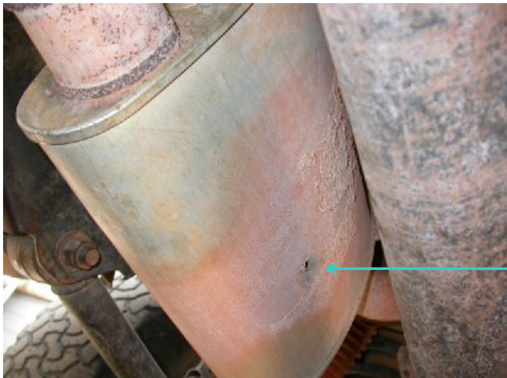
Figure 13 Location of leak in non-standard muffler box (arrow). This hole was used to locate thermocouple channel #3 in exhaust stream.
