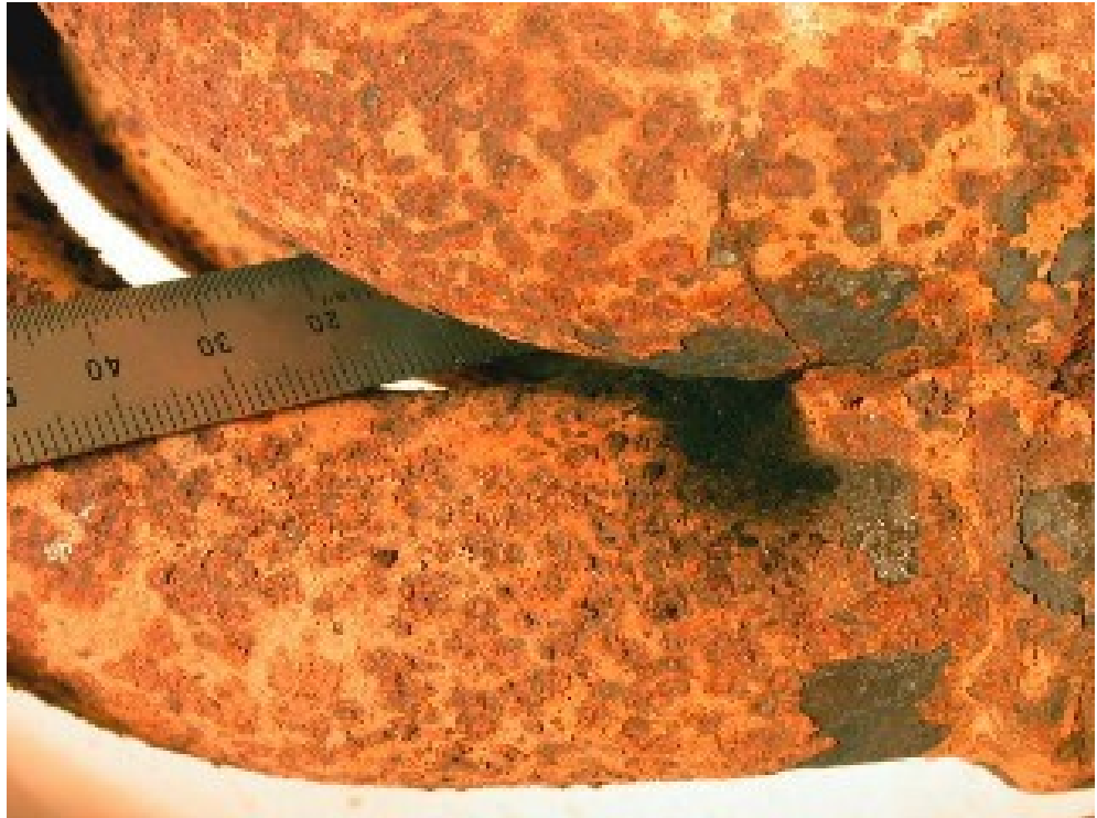
Figure 4 Detail of extractor tripoint connection showing carbon trail and cracked pipe (arrow). Note extensive corrosion.
