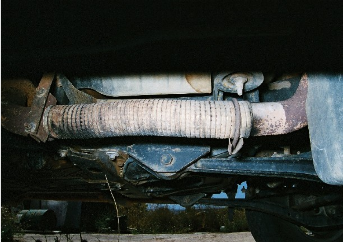
Photograph 53 Close-up view of the stainless steel after market flexi pipe fitted under the front right seat.
