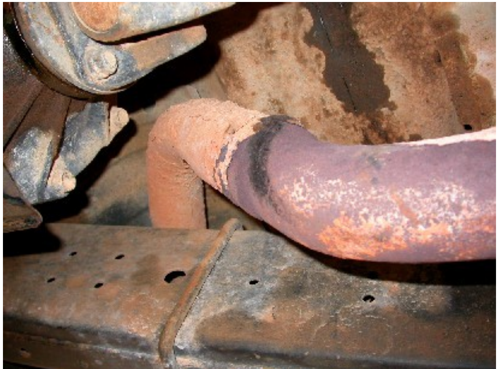
Figure 11 Detail of carbon trail associated with leak on main exhaust pipe adjacent to chassis rail. Thermocouple channel #4 was located on exterior of exhaust pipe at lower right of image.
