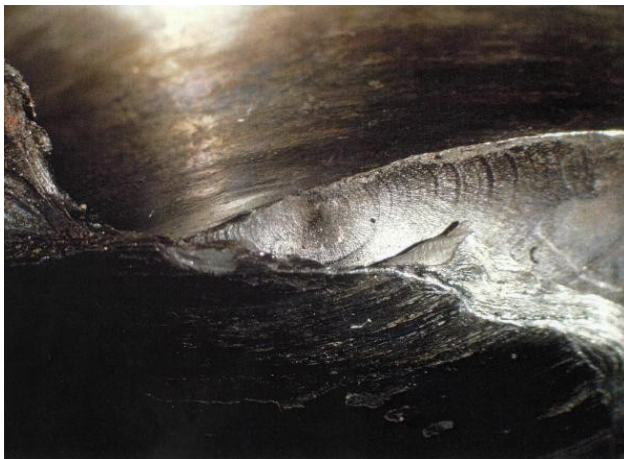
Mr McLean's photograph of MZK crankshaft fracture site Exhibit C221a
